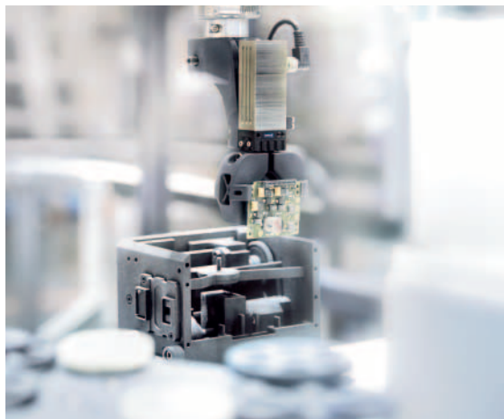
Use of an electric SCHUNK 2-finger parallel gripper EGP for precise handling of electronic components.
