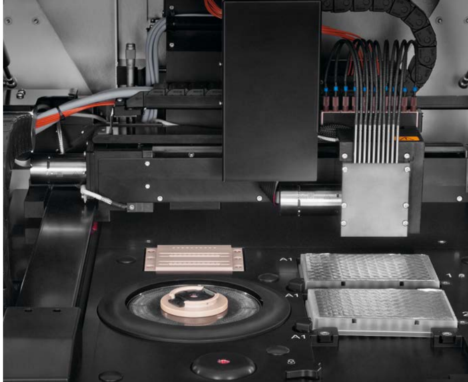
The high-precision control electronics with more than 3,000 position set points and low torque ripple ensure that the samples are positioned accurately on the CD, directly at the inlet of the respective channel.
