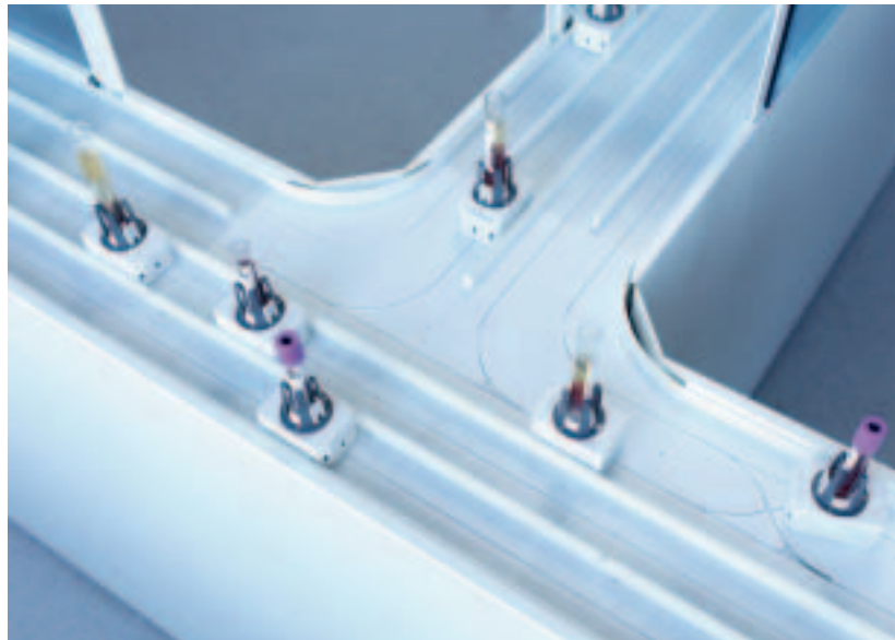
Highly flexible automatic sample distribution system: it transports each sample (specimen) individually, as this is the only way to achieve flexible, custom, and optimum organization of individual samples
