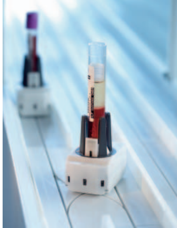
The track switches are set by the primary control system. Each track switch performs an average of 4,500 sorting processes per hour
