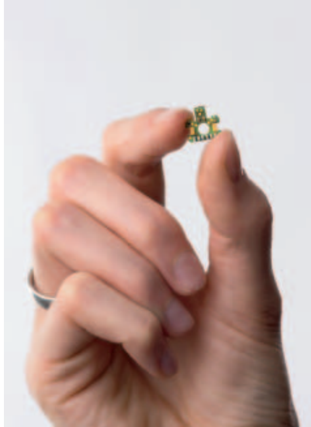
Hall sensor and electronics are housed in a single-chip off-axis component
